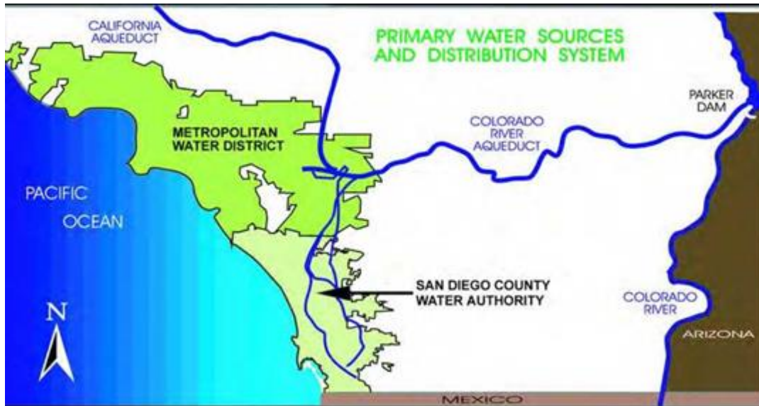
Figure 3-1 Imported Water Distribution
