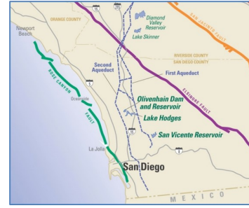
Figure 1 – Water Supply Pipelines Crossing Earthquake Faults
