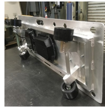
Underside of Cart Showing Motors and Angled Wheels
