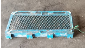
Prior Cart Used Inside Pipelines
