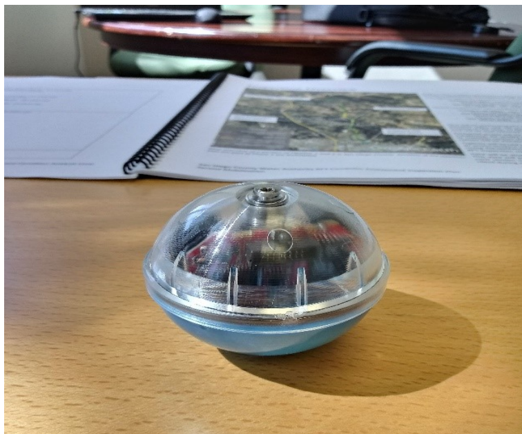
Acoustic leak detection ball, just 2.25-inches in diameter can be deployed in any sized pipeline 4 inches and above.
