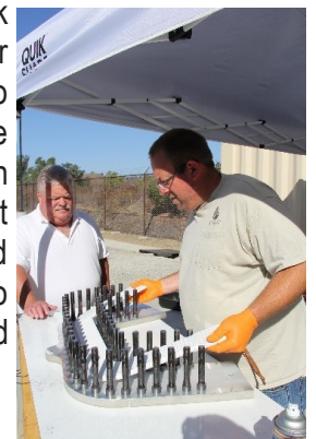
Wrapped bus bars within pressure mold
