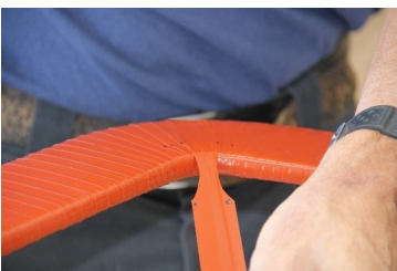
Precisely scalloped to minimize tape buildup at the inside corners
